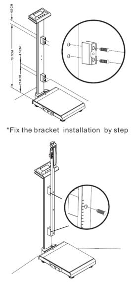
\*Screw the height rod on the bracket.
