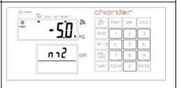
Press **[ENTER]** to save each pre-tare weight value into the memory, thus the scale instrument will make beep sound to confirm changes.
