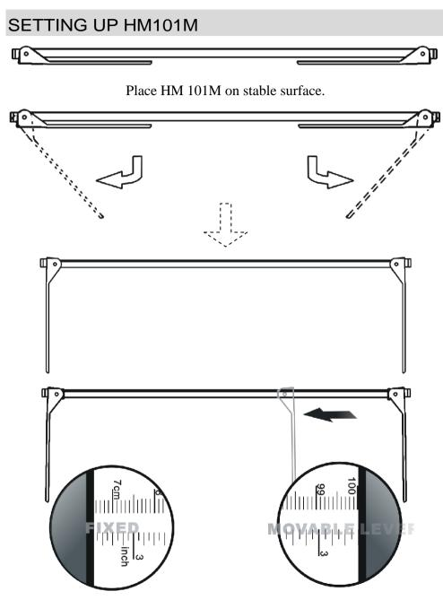
Measurement range is from 100mm to 1000mm
