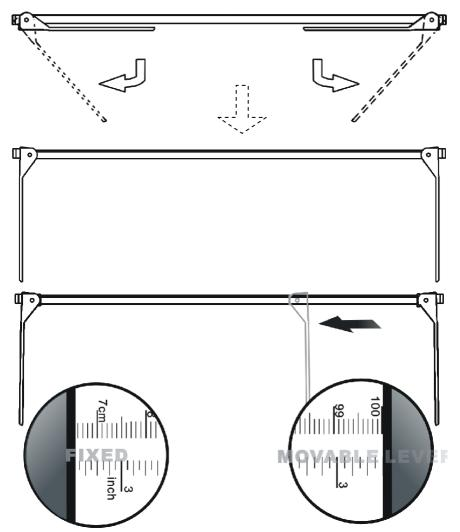
Measurement range between 100-1000 mm. Push head stopper to measure height.
