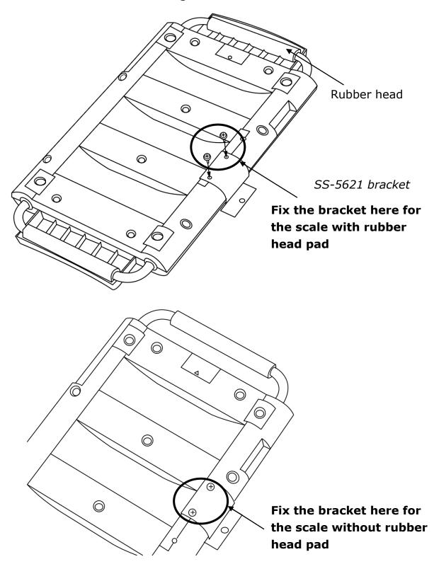
B. Assemble baby height rod with the bracket carefully until click.
