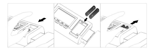
Installing battery AAA  $1.5V \times 2$  in battery housing next to LCD display
