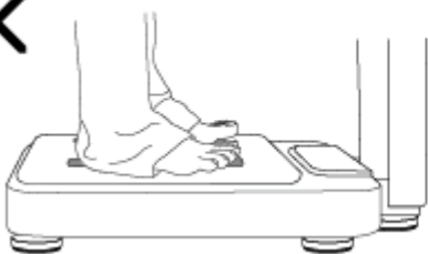
Heels are obstructed from full contact with rear electrodes due to clothing.
