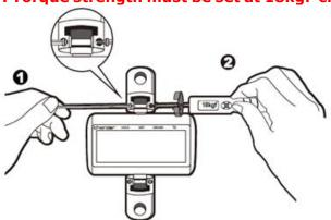
IMPORTANT: Nylock Screw must be secured from both sides (one side with screwdriver, other side by torque wrench). Nylock Screw will not tighten, and will simply rotate in place is counter-force from other side is not applied.
