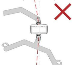
If any visual damage or bending is observed, do NOT use Lift Scale.
