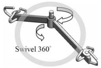
Even if the MHS2510I / MHS2610I Lift Scales with horizontally-rotating cardan joints are used, rotation should be conducted by the Patient Lift System, and not the Lift Scale, to minimize risk of damage to Lift Scale.
