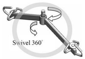
Even if the MHS2510I / MHS2610I / MHS2710 Lift Scales with horizontally-rotating cardan joints are used, rotation should be conducted by the Patient Lift System, and not the Lift Scale, to minimize risk of damage to Lift Scale.
