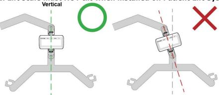
If Lift Scale is tilted and not completely vertical when installed, this will cause the joints of the Lift Scale to bend. This will eventually cause breakage once used enough times and subjected to enough weight, because force is being applied against joints in a way that they aren't designed to handle.
