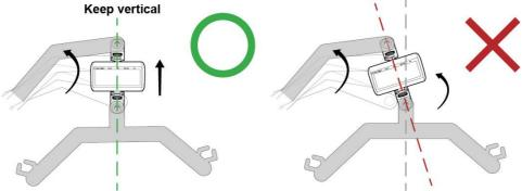
Even if Lift Scale is completely vertical when installed, if it is bent at any point in operation (ex: Patient Lift System raises patient to higher point for weight measurement), the same risk of breakage applies.
