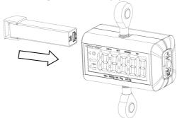
When power is low, please recharge the battery pack using the micro-USB port. When the port light is blinking **red**, battery is being charged. When the port light is stable **green**, battery is fully charged.
