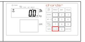
NOTE: Pre-tare weight must be under max capacity, otherwise screen will show 0.00 after **[ENTER]** key is pressed, and the operator will have to re-input pre-tare settings.
