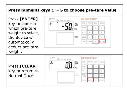
NOTE: Pre-tare weight must be under max capacity, otherwise screen will show 0.00 after **[ENTER]** key is pressed, and the operator will have to re-input pre-tare settings.
