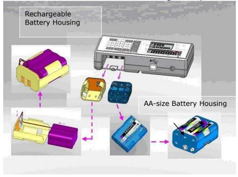
5. Install the battery housing into the compartment, and make sure the right side of housing pin is facing towards inside of the connecting position
