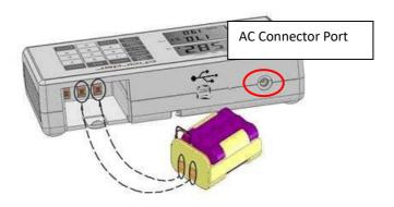
If prompt displays on the LCD, please charge battery promptly to avoid battery damage.
