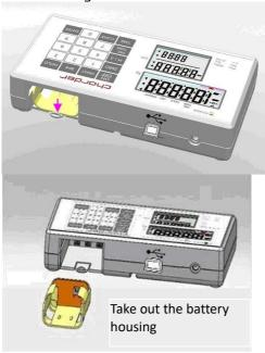
3. Use either rechargeable battery pack, or AA batteries
