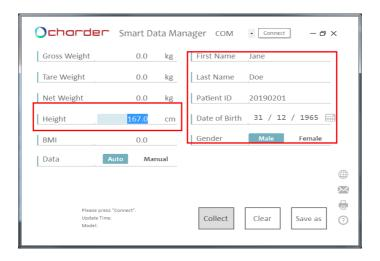
2. Conduct measurement. If **[Auto]** is selected, results will be transmitted from device to software automatically and displayed on the left of screen. If **[Manual]** is selected, user must press "Collect".
