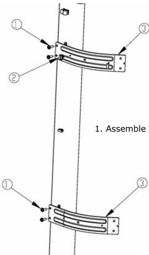
1. Assemble two brackets on the column
