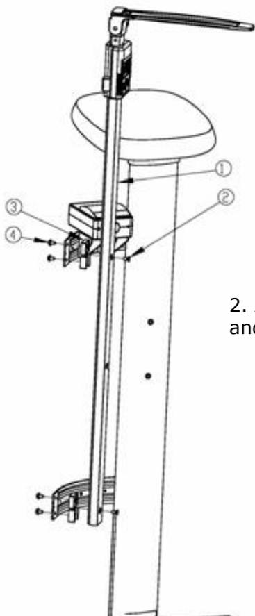
2. Attach Height Rod to bracket and tighten screws.
