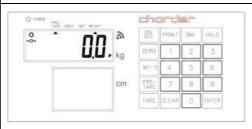
Manually enter numerical 0~9 key digits as the required pre-tare weight. For example: 5kg. Enter the key digits from left to right and then press **[ENTER]** to save it.
