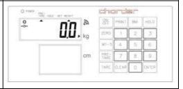
Press [CLEAR] key to correct digits in case if mistakes are made in typing; blinking zero will be shown on screen again.
