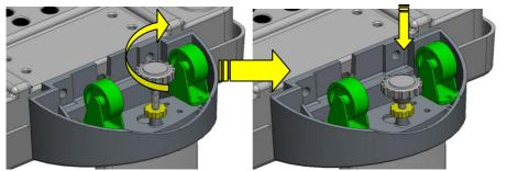
Note: rotate counter-clockwise to extend, clockwise to retract
