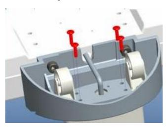
2. Ensure four adjustable feet and stability foot are at the same level before using the device. Rotate counter-clockwise to extend, clockwise to retract
