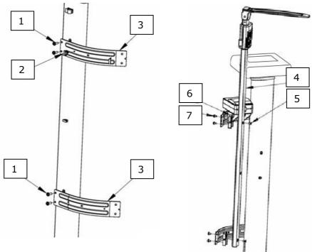
1. Attach brackets to column with round-head screws
