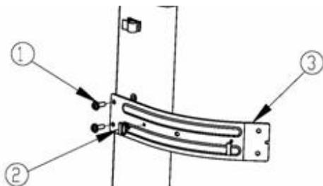
1. Assemble two brackets on the column
