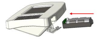
4. Close battery housing compartment cover. Turn on power to confirm that battery is correctly installed.
