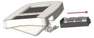
3. Place new battery pack into housing, and insert into indicator
