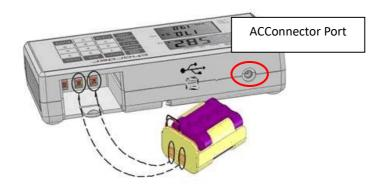
If **Lo** prompt displays on the LCD, please charge battery promptly to avoid battery damage.
