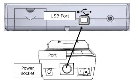
NOTE: Thermal printer needs to be powered by adapter
