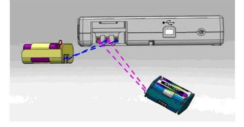
6. Slide back the cover to close the battery housing compartment. Turn on power to confirm that battery is correctly installed.
