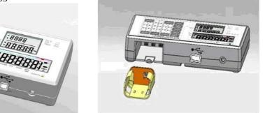
3. Use either rechargeable battery pack, or AA batteries
