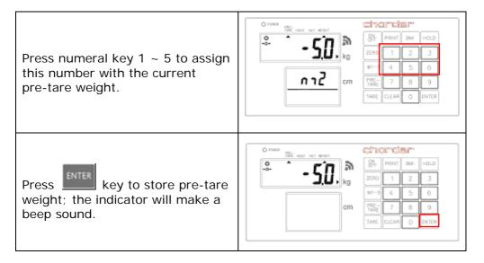
**NOTE**: Pre-tare weight must be under max capacity, otherwise screen will show 0.00 after **[ENTER]** key is pressed, and the operator will have to re-input pre-tare settings.
