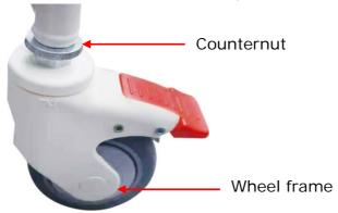
3. Adjust wheel height until air bubble on level indicator is level
