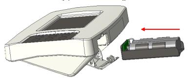
4. Close battery housing compartment cover. Turn on power to confirm that battery is correctly installed.
