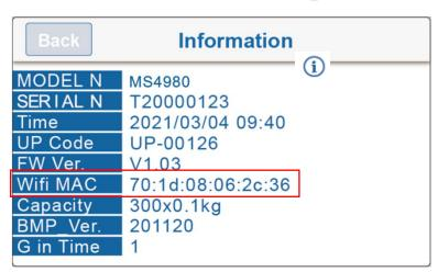
2. The "name" of the device's Wi-Fi Access Point will be "DP4800\_(MAC Address)" The default password to connect to the device is "00000000"
