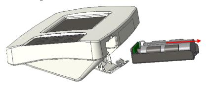
3. Place new battery pack into housing, and insert into indicator
