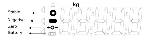
Stable symbol: Indicates that weight is stable.Negativesymbol: Weight under zero.Zero symbol: Weight is at zeroLow battery: Battery needs to be charged or replaced.
