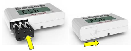
6. Turn on power to confirm that battery is correctly installed.
