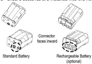
4 · Install the battery housing into the compartment, and make sure the right side of housing pin is facing towards inside of the connecting position
