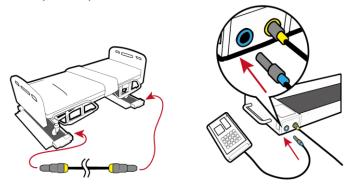
**Note**: connect both weight bridges to one another using weight bridge connecting wire. Connect indicator to weight bridge 2 (blue port).
