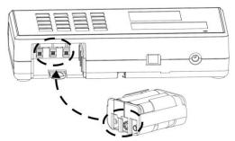
5 · Slide back the cover to close the battery housing compartment. Turn on power to confirm that battery is correctly installed.
