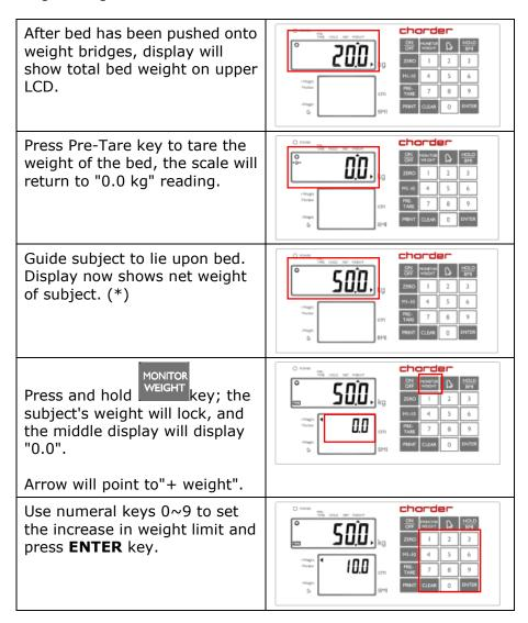
The lower display will begin blinking, pointing to the (-) weight limit. (\*\*). Use numeral keys 0~9 to set the decrease in weight limit. The minus (-) sign will appear in front of the weight decrease INN value. After setting the weight decrease value, press the **ENTER** key. (\*\*). Indicator will return to "0.0". **MONITOR** WEIGHT Press key to turn on the alarm. The blinking arrow pointing to sign means the Alarm volume is at maximum. To decrease volume level, press key again, and the
