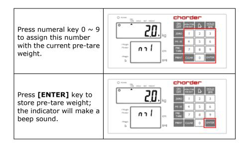
**NOTE**: Pre-tare weight must be under max capacity, otherwise screen will show 0.00 after **[ENTER]** key is pressed, and the operator will have to re-input pre-tare settings.
