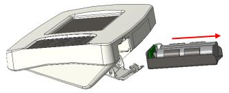
3. Remove battery pack from housing. Press down on tabs marked in red circles and push battery pack outwards (not entirely).
