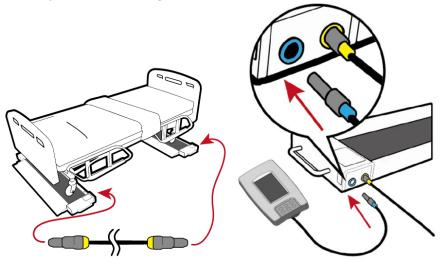
Yellow cable should be plugged into yellow port (for weight bridges)
