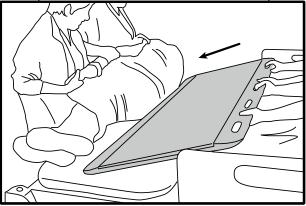
2. Help subject lie upon measurement platform. Conduct measurement (see Chapter V - Using Device).
