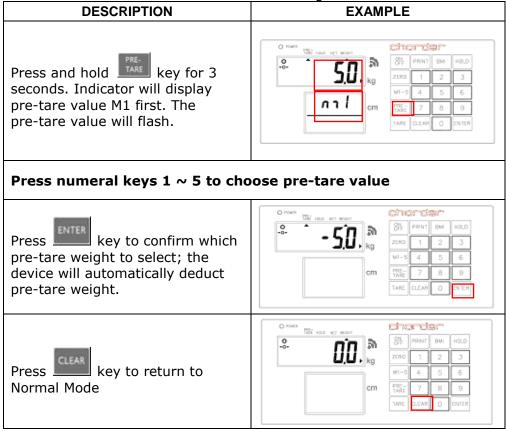
NOTE: Pre-tare weight must be under max capacity, otherwise screen will show 0.00 after key is pressed, and the operator will have to re-input pre-tare settings.
