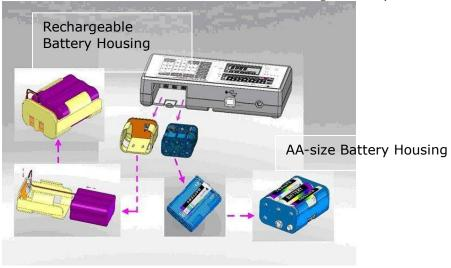
5. Install the battery housing into the compartment, and make sure the right side of housing pin is facing towards inside of the connecting position
