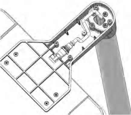
3. Route cable along gap in the column seat
