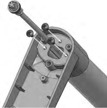
2. Secure column using three M4*0.7*15 screws
