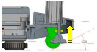
Ensure stability foot is retracted before using castor wheels
