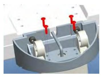
2. Ensure four adjustable feet and stability foot are at the same level before using the device. Rotate counter-clockwise to extend, clockwise to retract
