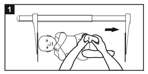
2. Use right hand to push foot stopper until it touches soles of infant's feet. You can also read measurement result from stadiometer. The height measurement result will automatically be sent to device indicator and display at the same time.
